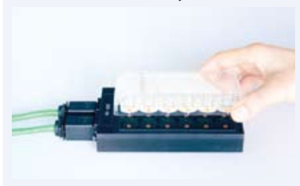
Figure 1. Online monitoring of DO and pH value in Keratinocyte cell culture with the SDR SensorDish® Reader by PreSens.
