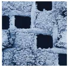
exciting the stainless steel mesh wires of a powder-screening machine by high-frequency, low-amplitude vibration to prevent apertures blocking has been used for over 25 years. The ultrasonic frequency is applied to the sieve mesh via an acoustically developed transducer (see Figure 3).
