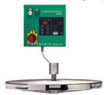
This breaks down the surface tension, effectively making the stainless steel wires friction-free and preventing particles both slightly greater and smaller than the mesh from blinding or blocking it. Screen blinding or blocking is a common problem when sieving difficult powders on screens of  $500\mu$ m and below. It occurs if either one or a combination of particles sit on or in an aperture of the mesh and
