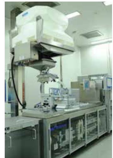
Figure 7: Matcon IBC loading a blister line
