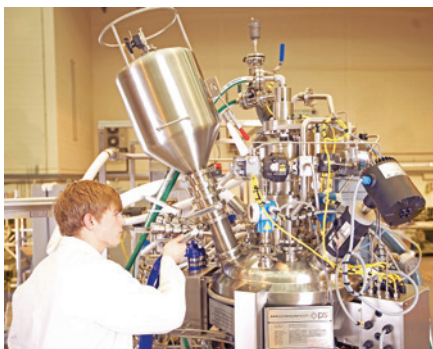
Image 3: MSR vessel with PAT and instrumentation
