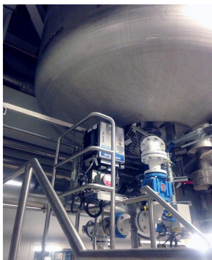
Figure 3. Installation of the METTLER TOLEDO ReactIR 45P system at the bottom of the Tosylfuranoside reduction vessel (15,000 L). Mid-IR operation is continuous 24/7.
