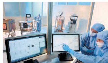
The real-time monitoring and prediction system, SIMCA®-online, constantly monitors processes to provide a continuous snapshot of the users' operations.
