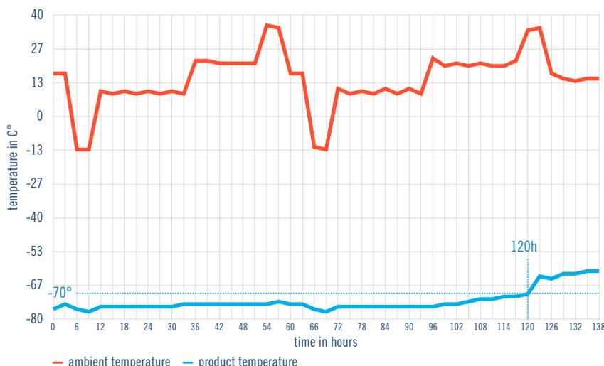
The PROTECT packaging system, when filled with dry ice, maintains a temperature of -70 °C for 120 hours. The ISTA 7D cold/hot profile was tested here. photo: eutecma
