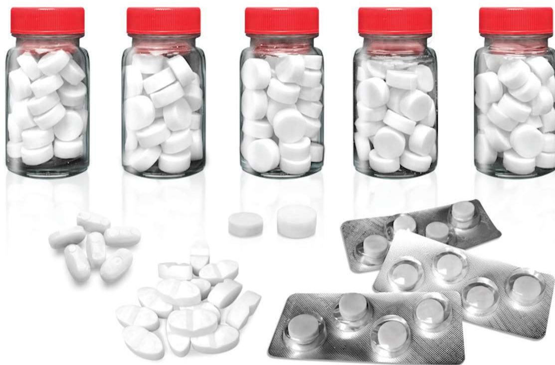
Moulded tablets obtained with the Extrusion-Moulding-Coating unit.
