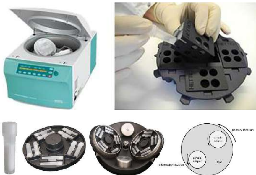
Figure 2: Dual centrifugation was used to expedite the development of an API nanoformulation
