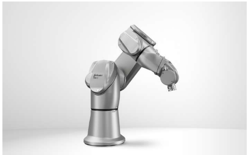
TX2-40 Stericlean+ is designed exclusively for use in isolators with an improved hygienic design on the covers and new FDA-compliant dynamic sealing on each joint
