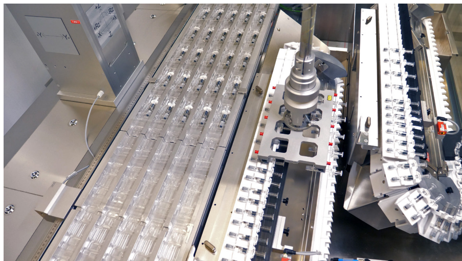
At the first robot station, a Stäubli TS2-60, equipped with a tenfold gripper, inserts filled syringes.
