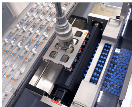
View of the gripper on the four-axis robot. Clearly visible: the various components with which each blister is filled.
