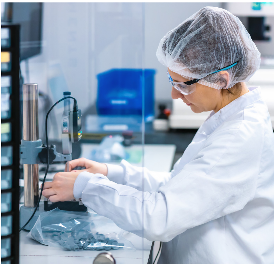
Figure 1: Functional Testing of Rubber Stopper Components
