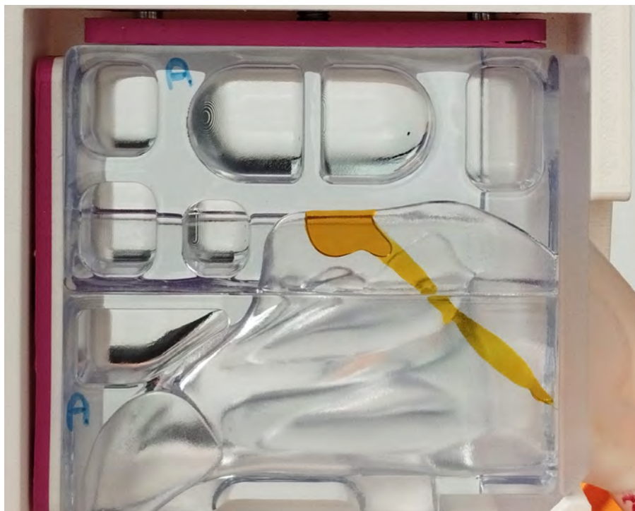
Figure 4 – Nemera CUBO nasal cast showing delivery of a coloured liquid formulation to the representative olfactory zone using the GST device with an automatic actuation, in a controlled experimental setting
