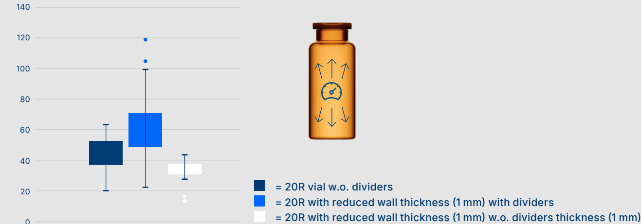
Figure 15: Strength comparison 20R vial vs. 20R vial with reduced wall thickness
